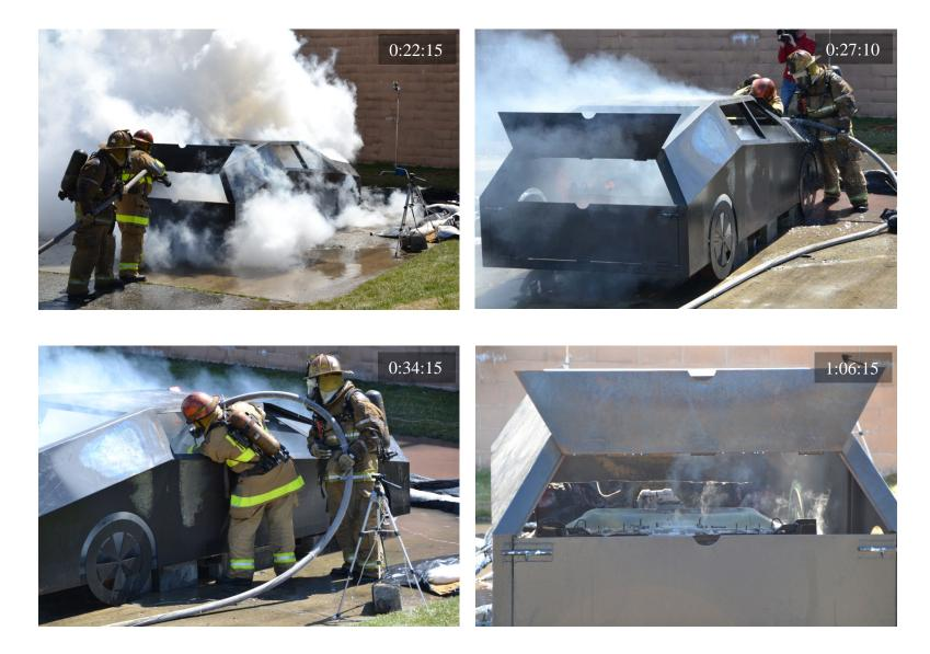
Figure 81 Test B2: suppression starts (top left); reignition and suppression (top right, bottom left); post suppression (bottom right)
