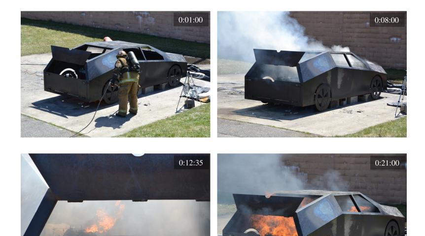
Figure 80 Test B2: ignition (top left); off gassing (top right); flames from fuse (bottom left); burners off (bottom right)
