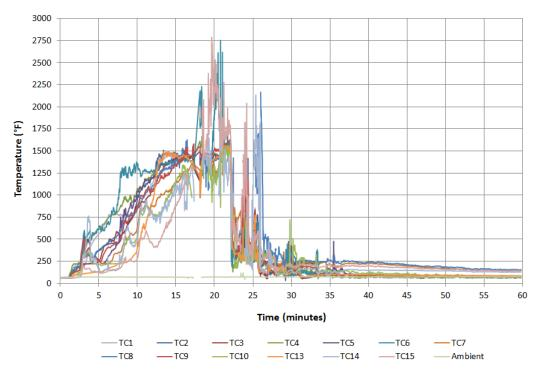
Figure 90 Test B3 TC plot
