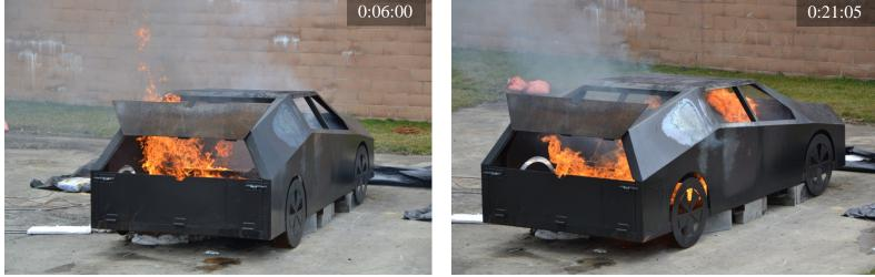
Figure 74 Test B1: ignition (top left); off gassing (top right); fully involved (bottom left); burners off (bottom right)
