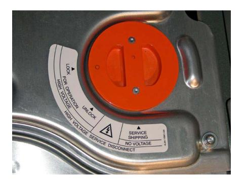
High-Voltage Service Disconnect Switch Shown in LOCK position. High-voltage system is STILL ACTIVE.
