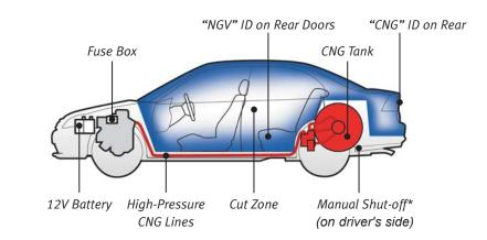
\* To access manual shut-off, reach between left rear tire and mud flap. Turn red handle to the right.
