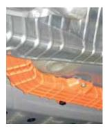
Electrical shield bolted to undercarriage
