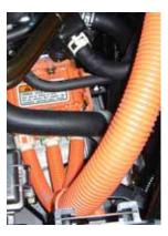
High-Voltage Cable Connection to Motor
