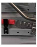
Thermal shield near hot exhaust
