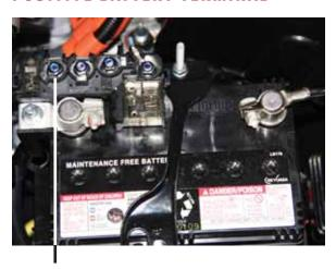
DC to DC Converter Cable Connection
