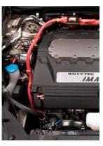
High-Voltage Cable to Accord AC Compressor
