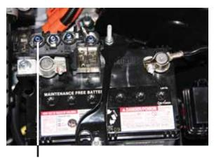
DC to DC Converter Cable Connection
