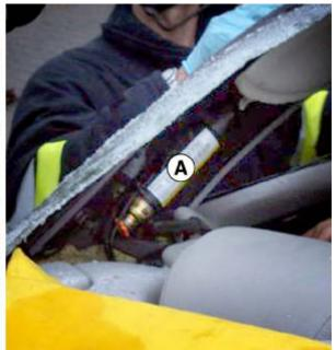
Compressed gas generator in the C-pillar!
