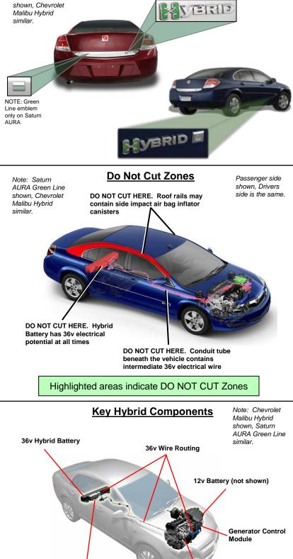
Hybrid Battery Disconnect Control Module
